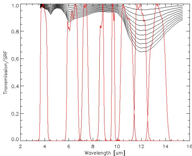
**Fig. 3. Transmittance spectra of ice layers of different thicknesses (black): 0.1 to 1.0  $\mu\text{m}$  layers (thickest layers have lowest transmittance) and Spectral Response Functions (SRFs) of Meteosat-8 infrared channels (red).**
