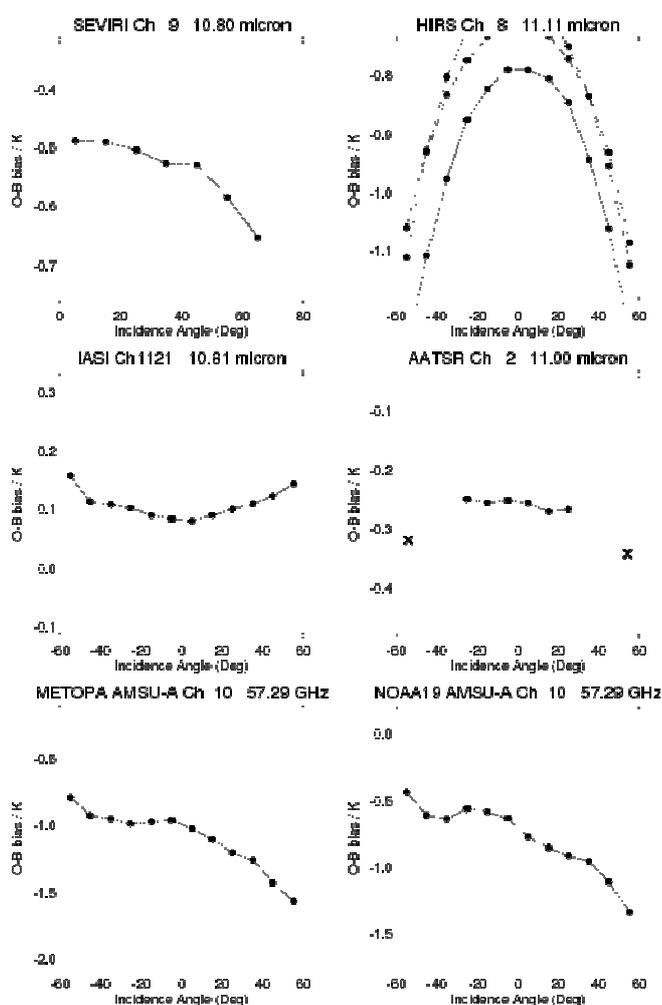
Figure 11. Plots of the mean clear sky bias for the 11 $\mu$ m channels of SEVIRI, HIRS, IASI, AATSR and AMSU-A as a function of incidence angle at the surface. The 3 lines on the HIRS plot correspond to data from Metop-A, and NOAA-17/19. The crosses on the AATSR plot correspond to the forward view. The data are over the ocean for 2010 except AATSR which is from Sept 2010 to Aug 2011.
