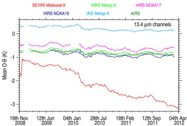
Figure 5. Plots of the O-B mean bias for the 13μm channels from SEVIRI (channel 11), NOAA-17, NOAA-19 and Metop-A HIRS (channel 7) AIRS (channel 355) and IASI (channel 434). All plots are just over the SEVIRI area (i.e. 60N-60S, 60W-60E) for clear sky ocean points.
