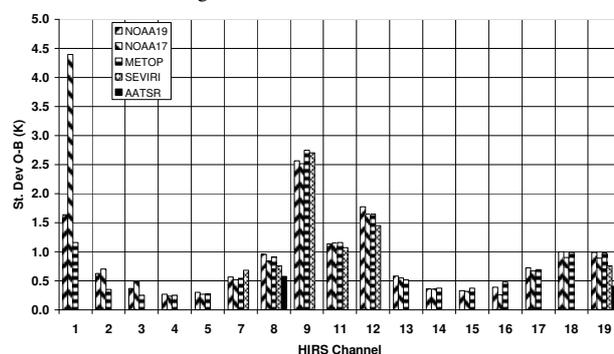
Figure 2. As for Figure 1 but the global mean standard deviation of the O-B difference for HIRS and common SEVIRI and AATSR channels.
