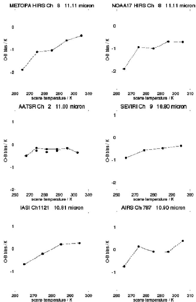
Figure 10. The changes in O-B bias for scene temperature for the 11 $\mu$ m window channels on HIRS on Metop-A and NOAA-17 (top panels), AATSR and SEVIRI (middle panels) and IASI and AIRS (lower panels). These are global clear sky statistics over the ocean for 2010 except AATSR which is from Sept 2010 to Aug 2011. The dashed line on the AATSR plot is for the forward view.
