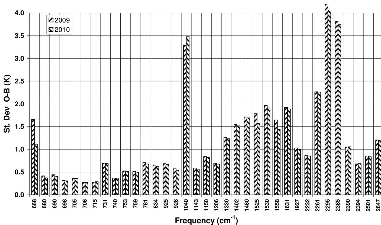
Figure 4. AIRS (top panel) and IASI (bottom panel) standard deviation of O-B for 2009 and 2010. The shortwave channels are for night-time only.
