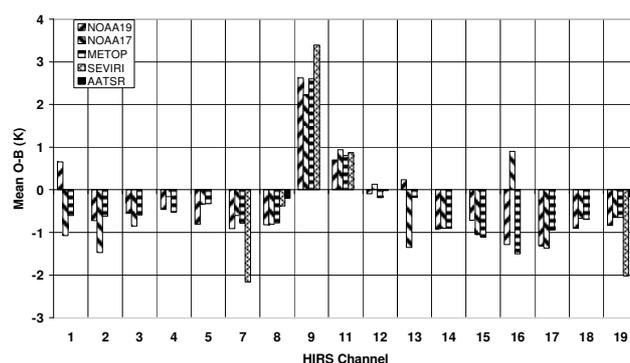
Figure 1. Global mean O-B biases of HIRS channels over the sea for 2010. The shortwave channels are only for night-time data. The corresponding SEVIRI and AATSR channel biases are also plotted for those channels which are common in wavelength.
