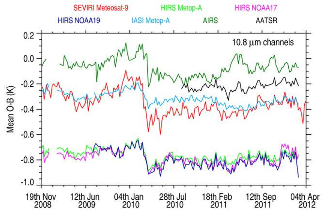
Figure 7. Plots of the O-B mean bias for the 11μm window channels from SEVIRI (channel 9), NOAA-17, NOAA-19 and Metop-A HIRS (channel 8), AATSR (channel 2), AIRS (channel 787) and IASI (channel 1133). All plots are just over the SEVIRI area (i.e. 60N-60S, 60W-60E) for clear sky ocean points.
