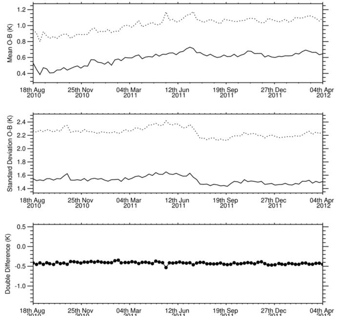
Figure 8. Plots of MHS upper tropospheric water vapour channel (3) from NOAA-19 (dotted) and Metop-A (solid). Upper panel shows the O-B global mean bias, middle panel the standard deviation of the difference and lower panel the double difference. All plots are for global coverage.
