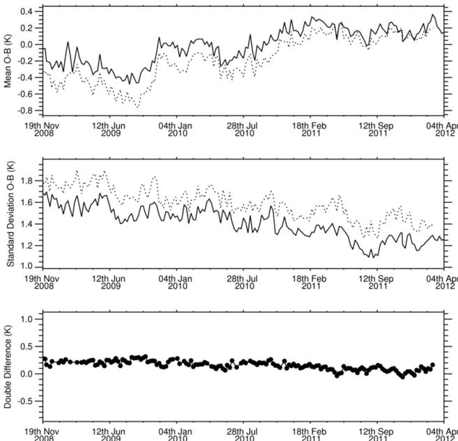
Figure 6. Plots of 6.2/6.7μm channels from SEVIRI (channel 5) as solid line and Metop-A HIRS (channel 12) as dotted line. Upper panel shows the O-B global mean bias, middle panel the standard deviation of the difference and lower panel the double difference. All plots are just over the SEVIRI area for clear sky ocean points.
