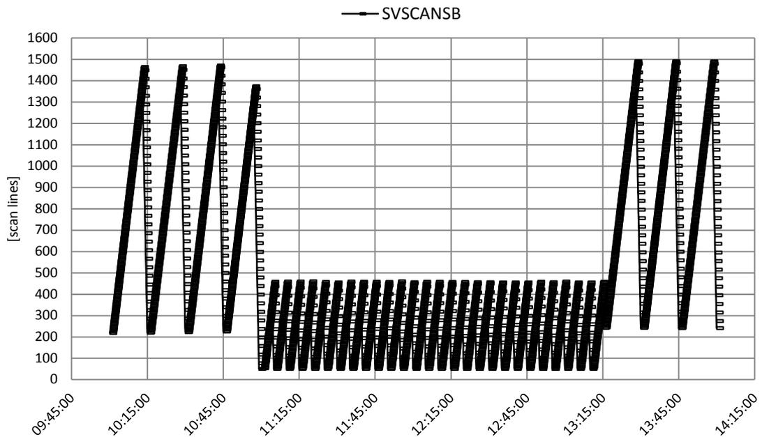
**Figure 8. SEVIRI scan mirror position**
