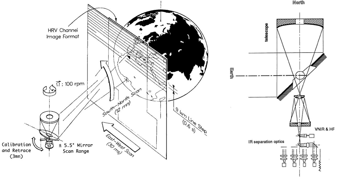
Figure 1. SEVIRI Earth imaging principle (left) and telescope overview (right).
