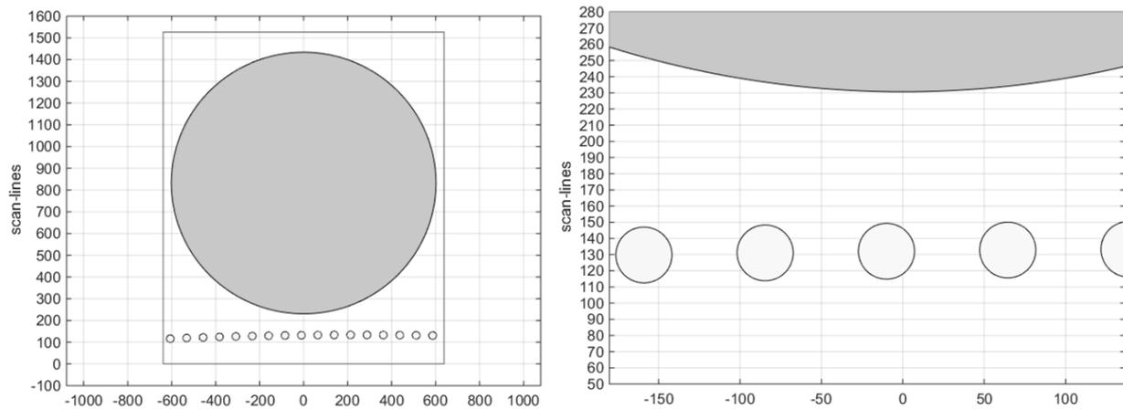
**Figure 6. Moon position during the transit on Saturday August 29<sup>th</sup> 2015 in SEVIRI nominal field of view.** *The image is zoomed-in on the right to show the ratio between Moon and Earth respect to the RSS image. As the RSS image is 410 scan lines above L0 (50), the Earth occupies exactly half of the RSS image.*
