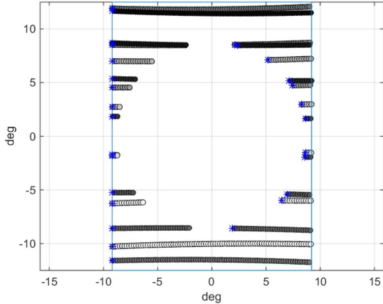
**Figure 5. Representation of the Moon intrusions in the SEVIRI FOV listed in Table 4. Results based on EUMETSAT Flight Dynamics predictions over the commissioning time frame.**
