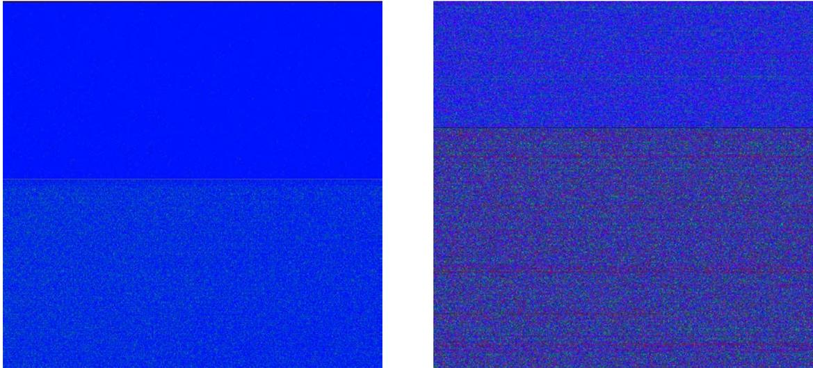
**Figure 9. Space Scan from Channels VIS 0.6 (left) and IR 12.0 (right).** Repeat cycles starting 09:15. The mean value is 51 counts, as expected. The noise is enhanced because of setting the MDU output gain  $q=1$ . The ColouringScheme is enhancing the noise. During retrace, in the upper part of the panel, the gain is reset to  $q=0$
