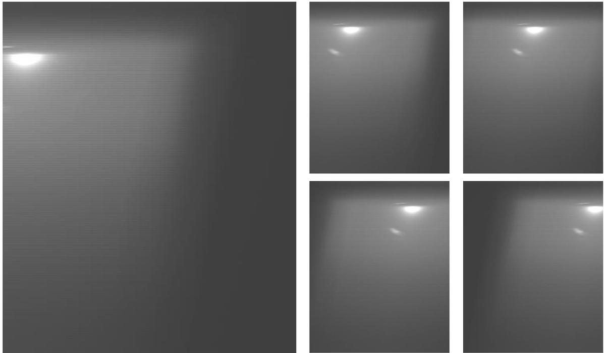
**Figure 11. Sun scanning images for the stray light characterization.** Sun transition in FOV during deep space scans for channel VIS 0.6. From left to right and top to bottom: repeat cycle starting at 10:30z, 10:45z, 11:00z, 11:15z and 11:30z, 27<sup>th</sup> August 2015.
