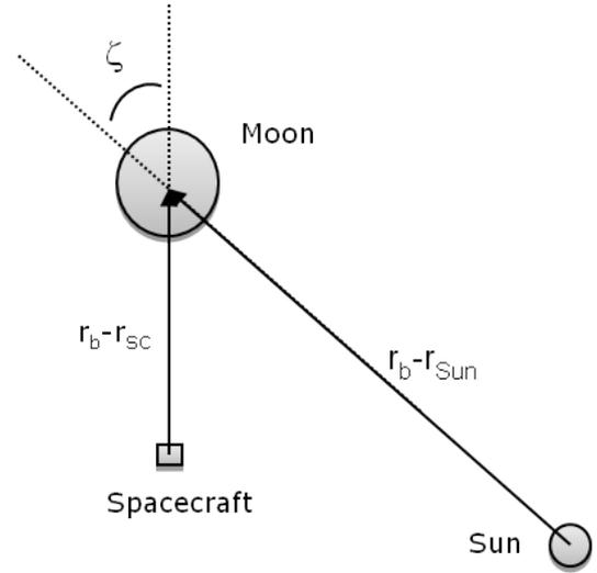
**Figure 3. First approximation of Sun lid percentage with angle between Sun and body.**
