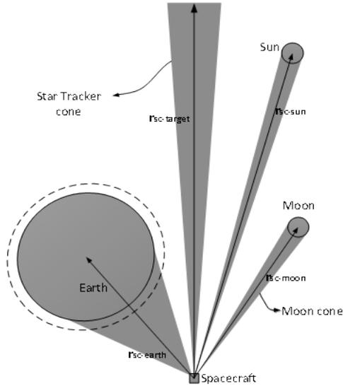
**Figure 2. Simplified geometric representation for determination of Sun/Moon/Earth intrusions in the instrument's Field of View.**
